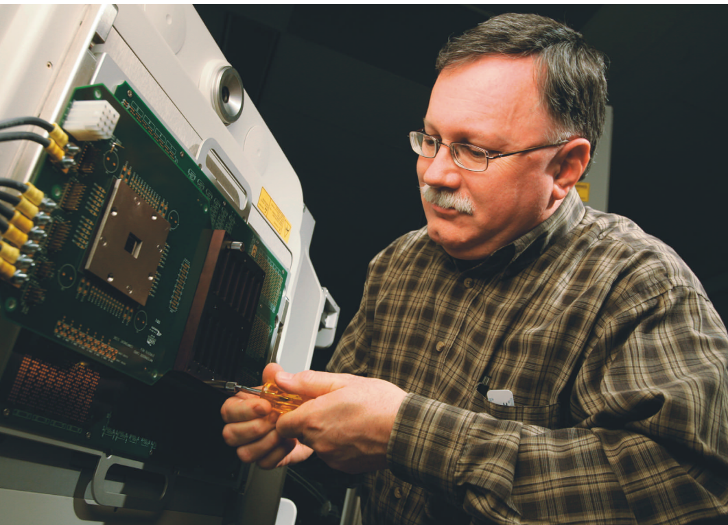
FIGURE 1. Rich Oldrey displays an Agilent 93000 load board, which interfaces 93000 pin electronics with daughter-card modules or probe rings that hold and provide electrical connections to devices under test within imaging tools.
