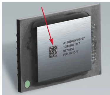
Fig. 1 The correct light facilitates the accurate reading of Data Matrix marks (red arrow) despite poor contrast against the reflective surface. Courtesy of Cognex.
